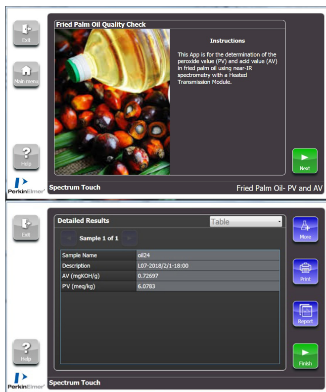
Figure 5. Spectrum Touch Workflow example for fried palm oil quality check.
