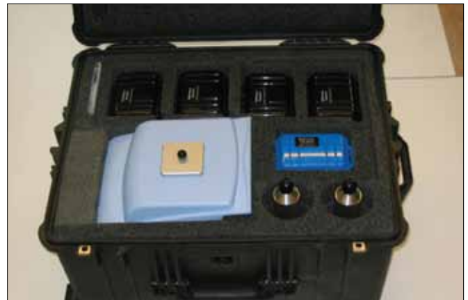
Figure 2. Kit includes Spectrum 100 sample pod, reflectance standards, supports for large panes and protective case.
