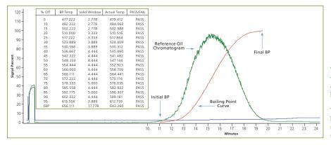
This is an example of a reference oil chromatogram with the calculated boiling point curve. Slices of the chromatogram are taken to determine the boiling point fractions.
