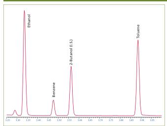
ASTM<sup>®</sup> Test Method, D3606, is an established method used to determine the benzene and toluene content in gasoline – originally developed to analyze gasoline that did not contain ethanol. Ethanol is now added to modern gasolines to improve combustion efficiency. The presence of large amounts of ethanol in samples may cause co-elution problems with benzene.
