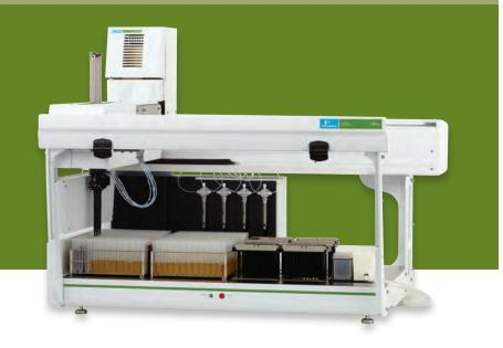
**Innovative Ultrasonic Liquid-Level Detector** allows unattended dilution of samples of different volumes, unaffected by viscosities, colors or ambient lighting.
