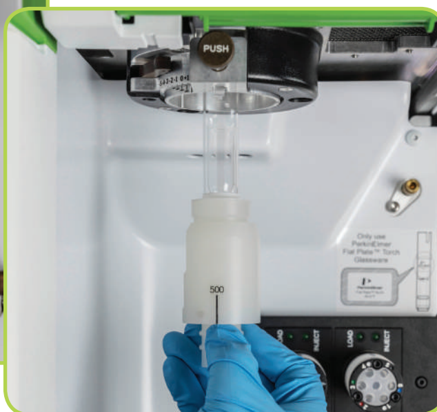
Installing a ZipTorch on Avio 500
