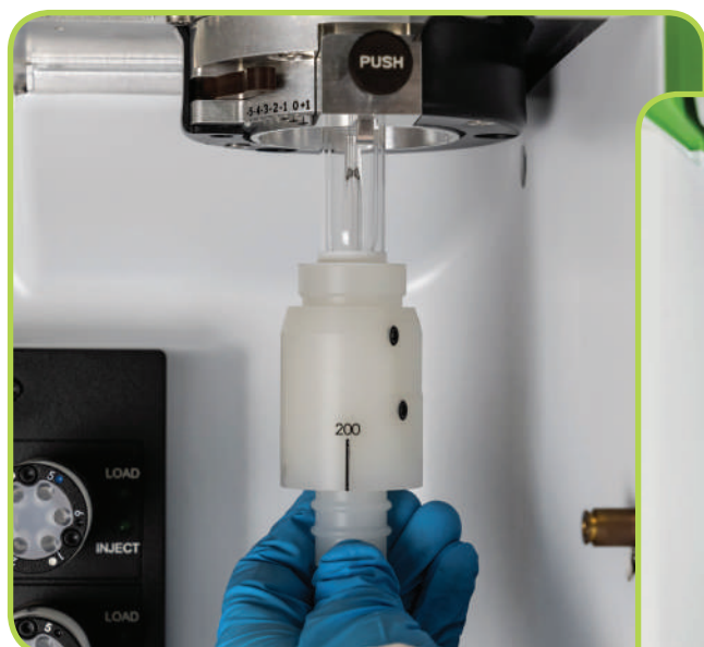
Installing a ZipTorch on Avio 200
