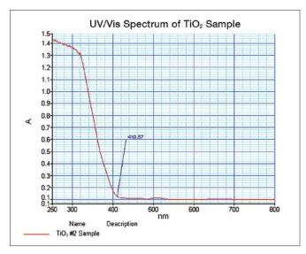
Figure 6. TiO<sub>2</sub> UV/Vis spectrum obtained in this work.
