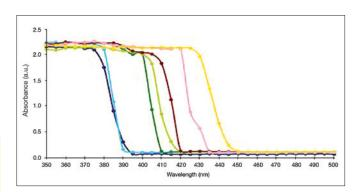
Figure 7. UV/Vis Absorption measurements for  ${\rm TiO_{2^-}}(X)~{\rm ZnFe_2O_4}$  nanocomposites.
