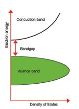
Figure 1. Explanation of band gap.
