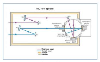
Figure 4. 150-mm Integrating Sphere Optical diagram.
