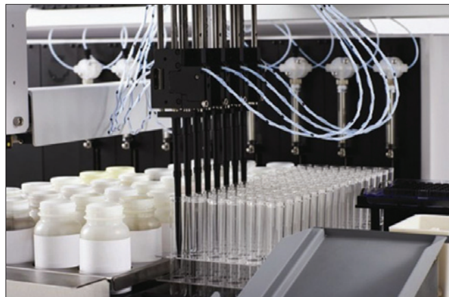
Figure 4. OilPrep 8 oil diluter with 8-tip Varispan pipetting arm and 1 mL disposable tips. A chemically resistant fluid path can accommodate up to eight independent system liquids, allowing multiple assays to be performed on a single automated platform. Custom racks, flexible deck layouts, and optional deck sizes (Mini, Standard, and Expanded decks) provide modular adaptation to unique protocols and vessel formats. Shown here: wide mouth sample bottles and 17 mm ICP-OES destination vials.
