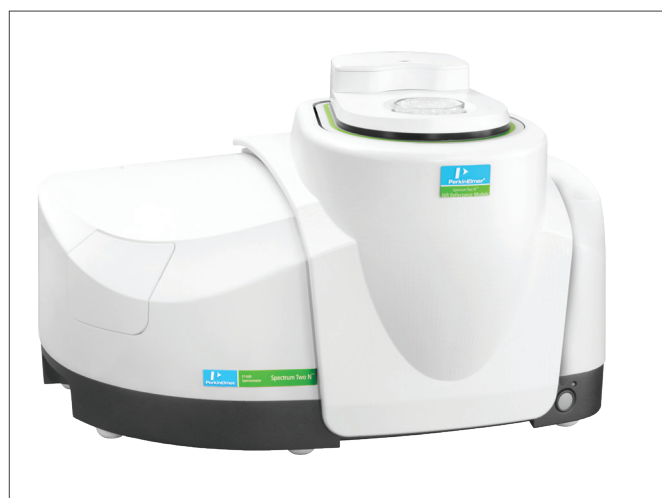
Figure 2. Spectrum Two NIR equipped with a Near Infrared Reflectance Module and sample spinner.
